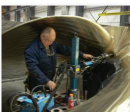
broken tap until the tap could be removed. With no damage to the threads a new tap was used to complete the threading process and the propeller was ready for shipment ahead of schedule.
